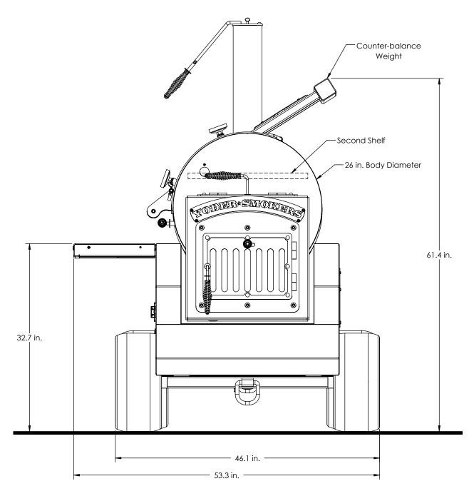
Overall Height: **72 in.** Overall Width: **53.3 in.** Overall Length: **92.8 in.** Total Weight: **1,750 lbs.**
