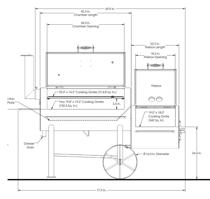
Overall Height: **58.2 in.** Overall Depth: **34.5 in.** Overall Length: **77.9 in.** Total Weight: **591 lbs.**
