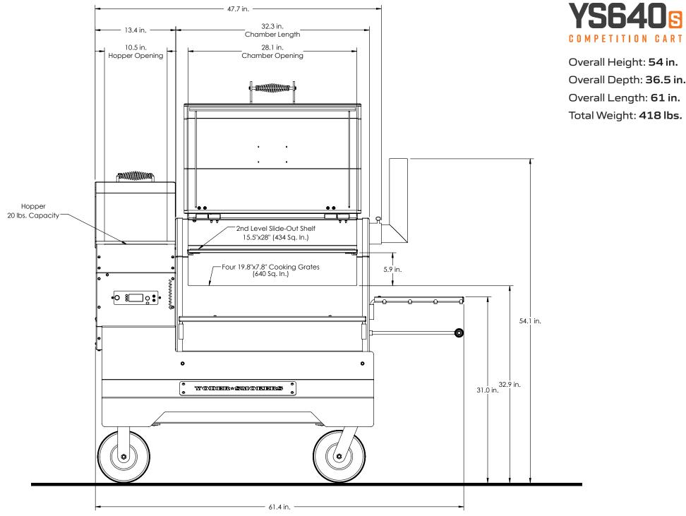
Overall Height: 54 in. Overall Depth: 36.5 in. Overall Length: 61 in. Total Weight: **418 lbs.**
