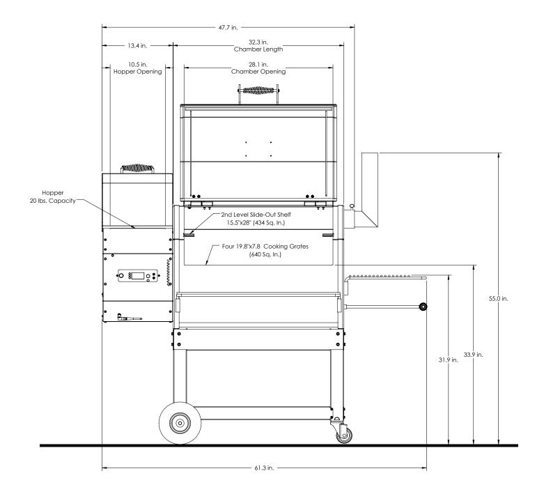
Overall Height: **55 in.** Overall Depth: **36.1 in.** Overall Length: **61.3 in.** Total Weight: **335 lbs.**
